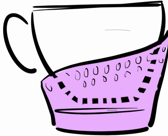
Figure 8. Thanks to the wave-inspired slope, FLOT can also be placed under cups with ears.
